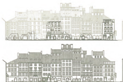
图 3: 插图展示了市场广场的立面形态。在上图中, 深色表示清除瓦砾后核定的建筑遗迹, 背景的浅灰色为战前的测绘图。下图是重建项目的设计图。(波兰建设部档案) Figure 3. Illustrations show the Market Square frontages. In the top elevation, the dark colour indicates remains of houses assessed after the removal of rubble, against the background of the pre-war survey, which is in light grey. The bottom elevation is a drawing for the reconstruction project design. (The archive of Polish Architecture Department - ZAP)
